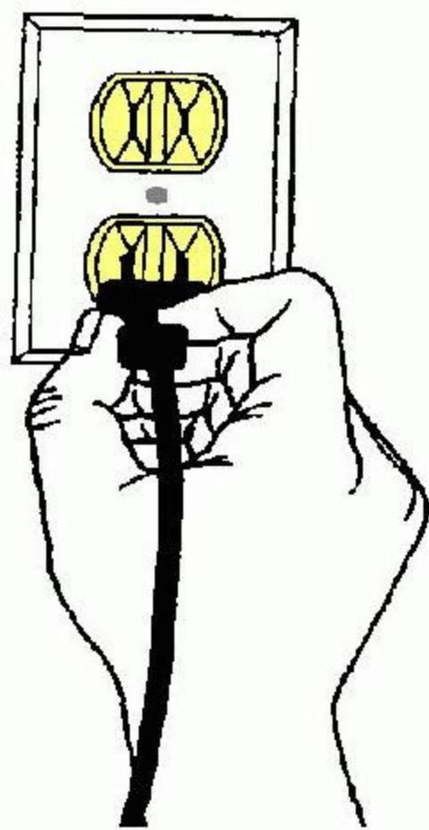
like a water faucet, you will receive a shock. If the appliance is plugged into an outlet protected by a GFCI, the power will be shut off before a fatal shock would occur.
